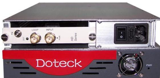
**One slot, built-in power supply**
